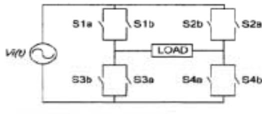
Fig 4.2 Single-phase matrix converter circuit configurations at load
