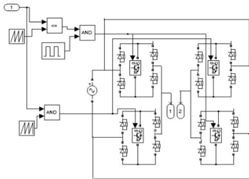
Figure 6.3 Subsystem 2 of the Closed loop DVR with a matrix converter
