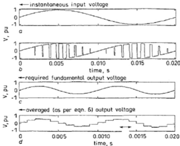
Fig 4.3 Input, Output, required output and averaged output wave forms
