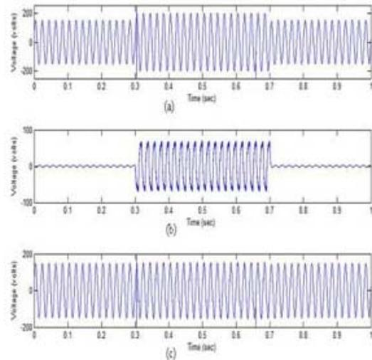
Figure 6.5 Response of RMC based DVR to a voltage swell
