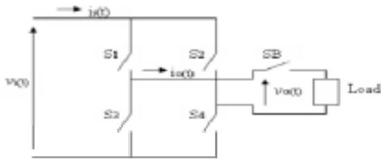
Fig 4.1 Single-phase matrix converter circuit configuration at no load
