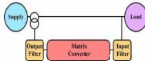
Figure 2.2 Matrix converter based DVR.
